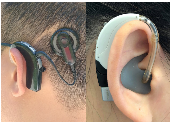
On the left is a cochlear implant and on the right is a hearing aid.
